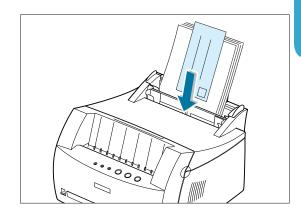
3 Adjust the guide to the edge of the envelope stack.
